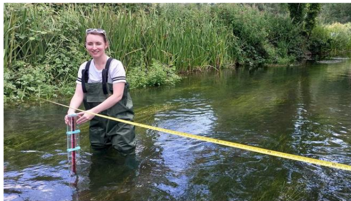
Sophie measuring flow depth with the TVHR
