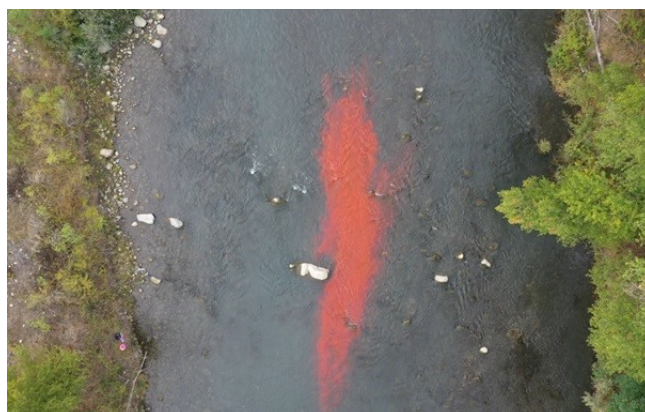
Tracer injection in the Durance River, La Saulce (25/09/2019)
