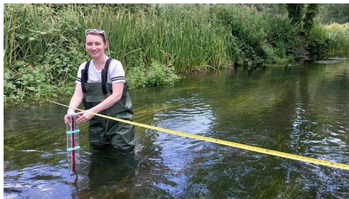
Sophie measuring flow depth with the TVHR
